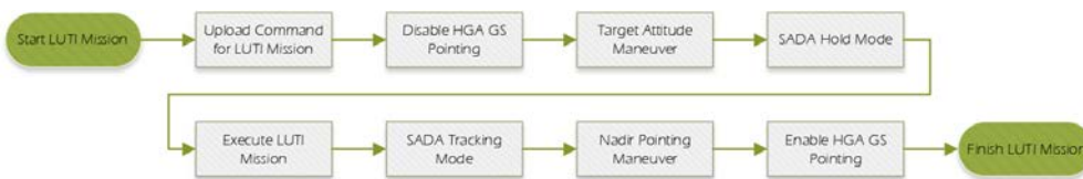
Fig. 12. LUTI mission operation flow. All LUTI mission commands are executed by absolute time commands. The mission commands for a day are planned and uploaded every day. LUTI, lunar terrain imager; HGA, high gain antenna; SADA, solar array driving Assembly; GS, ground station.
